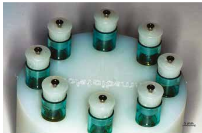
Figure 2. Centrifugation of the test tubes with Immediateload implants along with CGF or the Liquid Phase of CGF (LPCGF) by Round Up (Silfradent srl, Forlì, Italy).
